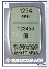
with the anti-collision system disabled and equipment in the CRITICAL zone, the buzzer sounds continuously.
