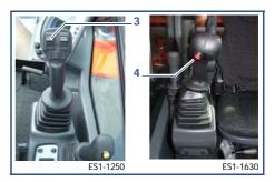
3 - while pressing the roller the automatic hold can be activated by pressing the red button (4) under the joystick, so the control will remain on without having to keep it pressed up; the automatic hold for the oil flow to the equipment can be activated at any stage of the roller travel, in this way making it possible to provide a partial flow and keep it constant at the required level. When the automatic hold is activated the relevant light on the dashboard comes on (5).
