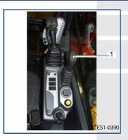
An indicator light on the dashboard will light up when the system is engaged. The system can be engaged either at standstill or while in motion. Pressing the activation button again will disengage the system, and the driving speed automatically reverts to the minimum.
