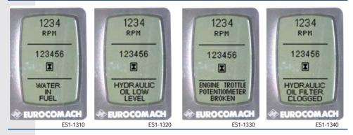
If the message "ACCELERATOR POTENTIOMETER BROKEN" appears the engine automatically cuts its speed down to 1400 rpm to prevent any irreversible damage.
