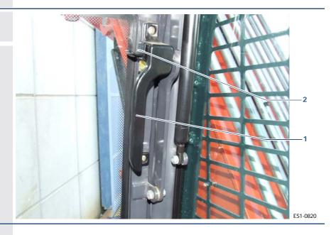
The windshield can be lowered by following the same procedure in reverse order until the locking "click" is heard. At this point the windshield will be completely closed.
