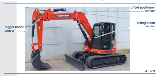
Together with the control box, these constitute an "Automatic Anti-collision System", the purpose of which is to guarantee operator safety, preventing the working equipment from accidentally colliding with the cab.
