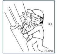
lines. Pressurised fluid leaks may be invisible. **NEVER** use your hands to check for leaks. Use a piece of cardboard or paper for this purpose. Wear gloves to protect your hands from any oil splashes.
