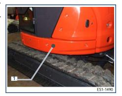
Anyone wearing a pacemaker, should check that the communication antenna (1) is located at least 30 cm from the pacemaker as the radio waves could exert a negative action on the way it works.
